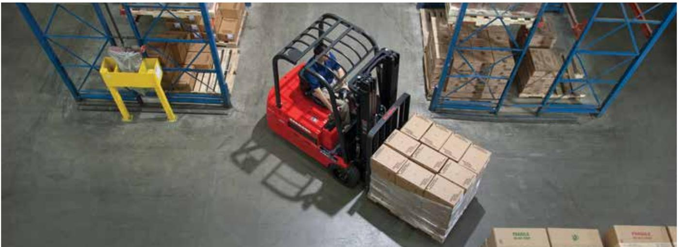
➤ On the Model 4450, dual AC drive motors and intelligent steering control deliver improved maneuverability and tighter turns.
