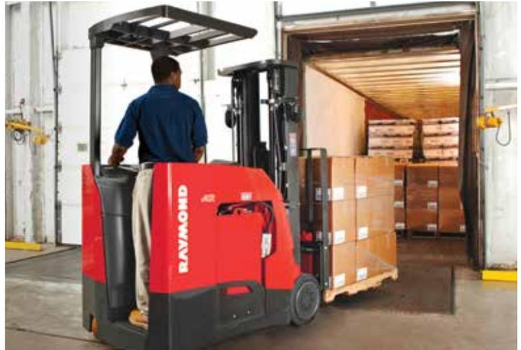
➤ Dual drive and steer wheel design allow one wheel to counter-rotate during turns to provide greater maneuverability.
