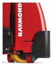
The heavy-duty optional bumper guard further absorbs and diffuses impacts from the frame and components.
