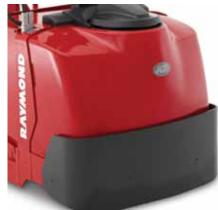
The heavy-duty optional bumper guard further absorbs and diffuses impacts from the frame and components.
